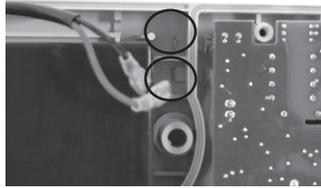
7. Dismount the wires from the batteries
