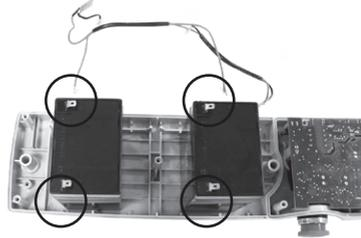
8. Replace the batteries by same type (LINAK A/S part number BA0CBJH00 (2 batteries with 1 wireharness)) OR as described in the section "Battery information".
