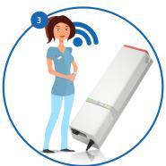
Release key and magnet and move closer to the LIFT50 $^{\text{TM}}$  until buzzer frequency change from slow to fast.
