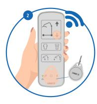
Enter Direct Pairing Mode by activating key 1 and magnet in 3 seconds.
