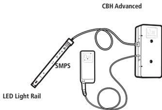
Connect the LED Light Rail to the CBH Advanced and add light under your bed design. Control the light via the standard hand control or the Bed Control App.
